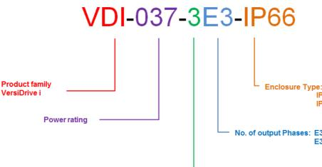
Enclosure Type: No Text = IP20 IP66S = IP66 switched IP66 = IP66 un-switched
