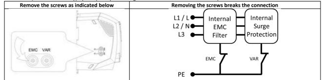
The VersiDrive i E3 product range has input supply voltage surge suppression components fitted to protect the drive from line voltage transients, typically originating from lightning strikes or switching of high power equipment on the same supply.
